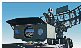
Optoelectronic head mounted on upgraded anti-aircraft missile combat vehicle PRWB OSA
